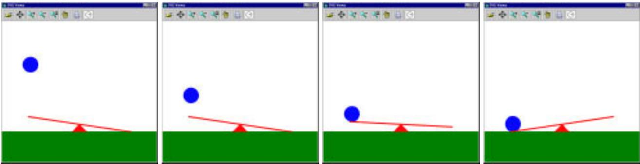
Figure 9: CSSVG animation of a ball falling towards seesaw. The position of the ball is directly related to time, and the seesaw moves because of constraints describing its behavior.
